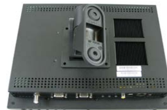
3. Attach the new 75mm x 75mm VESA-compliant mounting device or stand to the display.
