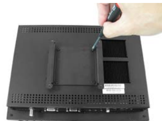
1. Unscrew the four screws attaching the 100mm x 100mm VESA-compliant adapter to the display, then remove the adapter.
