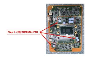
(c) Top side of PCBA – Remove shielding and thermal pad.
