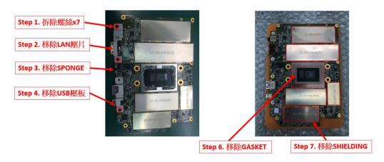
(b) Bottom side of PCBA – Remove thermal pad
